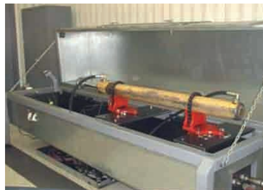
High pressure hydraulic leakage testing
