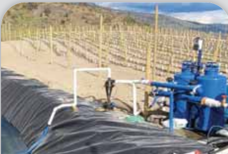
Hydro Cyclone filtering out sand in a vineyard irrigation system
