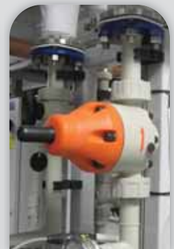
ChemFlare™ system with PFA tubing and fittings and PVDF back pressure/relief valve on medical DI water
