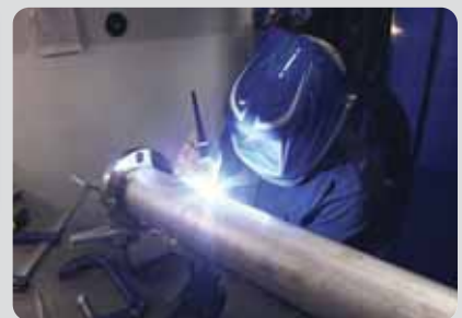
TIG Welding for fabrication of shaft extensions
