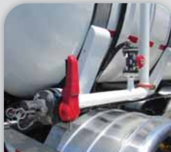
PVC butterfly and diaphragm valves on fibreglass tanker trucks hauling corrosive chemicals
